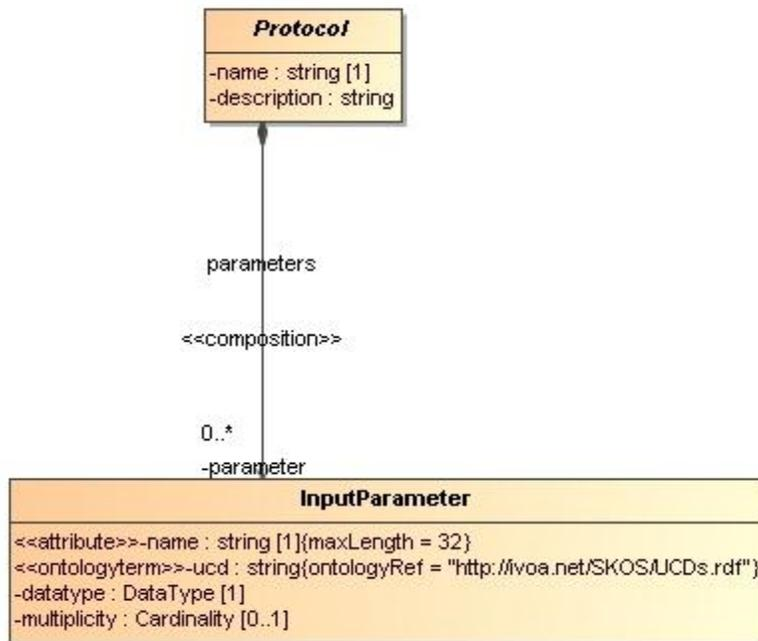
**Figure 24:** The line with the filled diamond on one end and an arrow on the other indicates a (parent-child) composition relation, or collection, between the parent, on the side of the diamond; and the child, on the other side.
