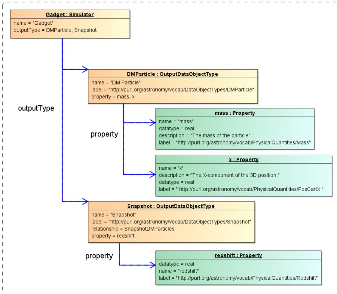
**Figure 5** Example instance diagram showing a Simulator with two output types, "Snapshot" and "DMParticle", each with properties. Note the SKOS concepts used in the label attributes. These may not (yet) exist in the corresponding vocabularies.
