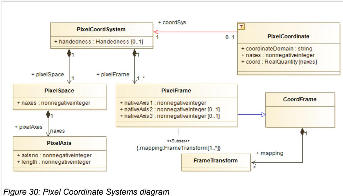
Figure 30: Pixel Coordinate Systems diagram
