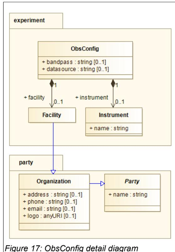
Figure 17: ObsConfig detail diagram
