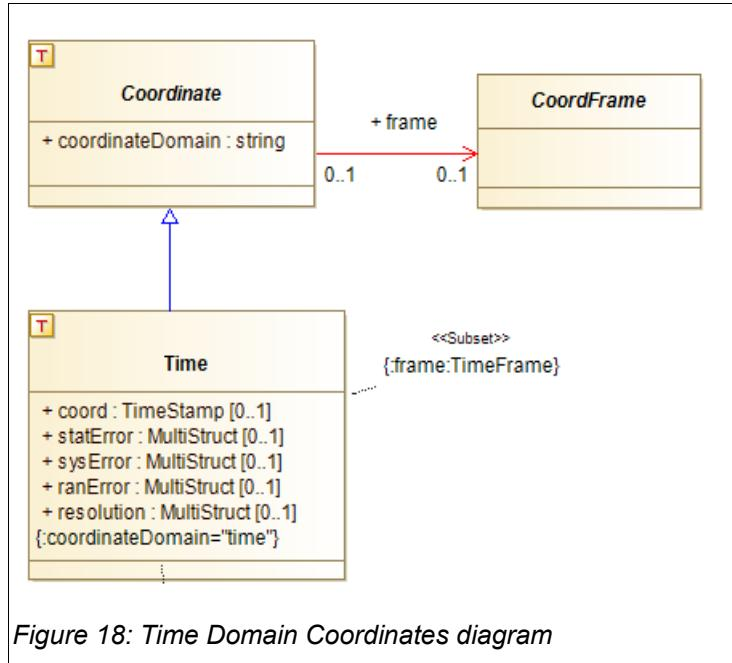
Figure 18: Time Domain Coordinates diagram
