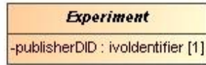
Figure 13: A Class is a rectangular box, with the name of the class in boldface.
